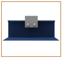
**Step 3:** Fasten clamp on side with 2 blind rivets.
