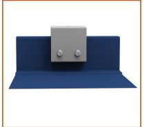
Step 3: Fasten clamp on side with 4 blind rivets.
